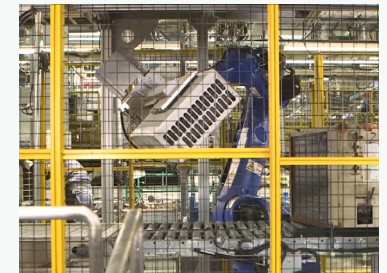
Machine to turn over air conditioner outdoor units at PETECK
