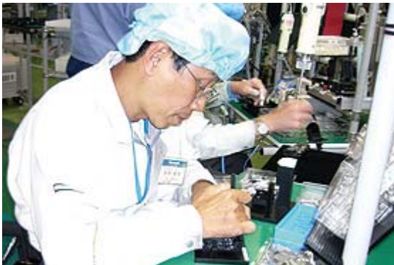
Mr. Kimura at work, assembling LSD parts of a video camera
