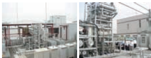
Verification test facility using solvent extraction for PCB polluted soil
