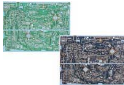
Previous printed circuit boards(up) Halogen-free printed circuit boards(down)
