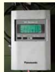
Measuring the energy consumed by equipment using a WH monitor made by Panasonic Electric Works
