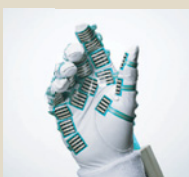
Gloves with pressure sensors used to measure grip pressure
