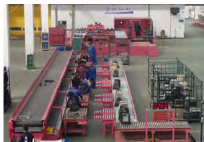
TV disassembly line in the new recycling company
