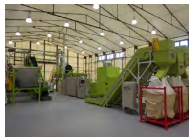
Near-infrared simultaneous sorting machine for three types of resin at CETEC
