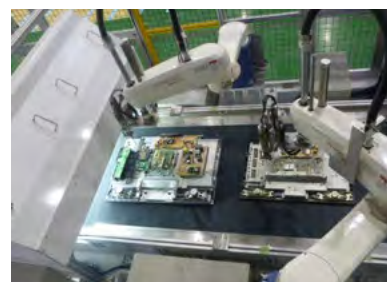
Automatic screw remover for flat screen TVs at PETECK
