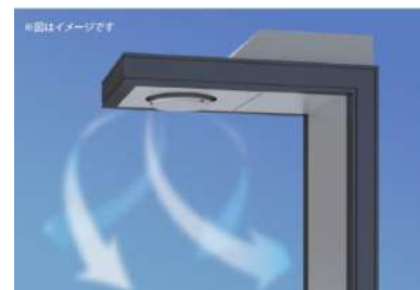
Air curtain creating dome-shaped cooling space
