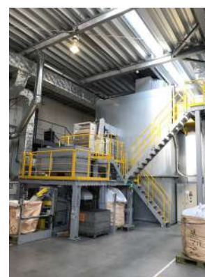
Compact crushing and sorting system for heat exchanger of air conditioner in PETECK
