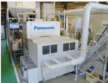
Near-infrared sorting machine that can sort three types of resin simultaneously
