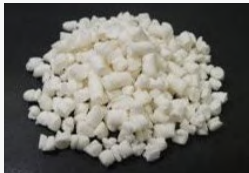
Cellulose fiber composition materials with a biomass content of 90% or more
