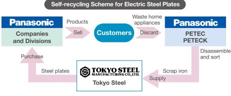
Specifically, scrap iron from home appliances collected and treated at PETEC and Panasonic Eco Technology Kanto Co., Ltd. is supplied to Tokyo Steel, where the scrap iron is processed into electrical steel plates.<sup>16</sup> We procure the recycled steel plates and utilizes them in products. Discussions with Tokyo Steel commenced in 2010, and we have worked together since then to improve the quality of recycled iron to a level sufficient for production use, as well as developing
