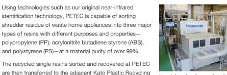
Near-infrared sorting machine that can sort three types of resin simultaneously
