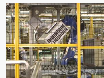
Machine to turn over air conditioner outdoor units at PETECK
