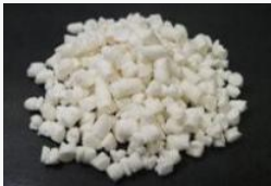
Cellulose fiber composition materials with a biomass content of 90% or more
