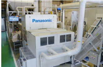
Near-infrared sorting machine that can sort three types of resin simultaneously
