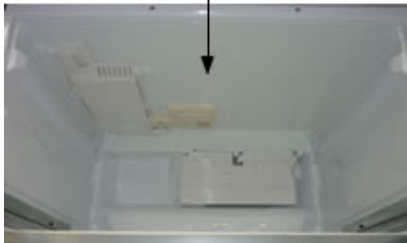
Vegetable chamber sealing plate inside refrigerators
